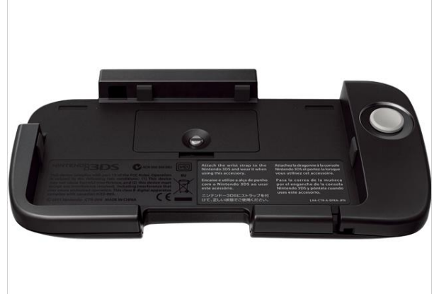
Figure 9. Circle pad pro contains an extra joystick for N3DS. The data is transmitted via IR. [12]
