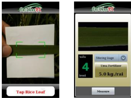
Figure 4: Screenshots taken of the “BaiKhao” app. The application controls the camera of the mobile device to take a picture of a rice leaf in a white reference paper (left), and then internally processes it to determine the color levels of the leaf and then estimate the amount of nitrogen fertilizer recommended (right).
