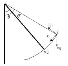
In order to study easily the behavior of the attraction, we are going to suppose that its movement is the same of a pendulum.
